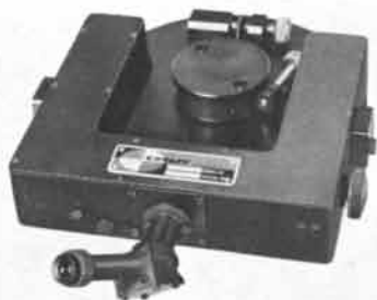
unisec measures angles accurately in missile-controlling submarines
