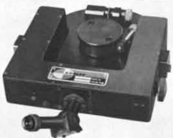
unisec is used to measure azimuth in the newest surveying equipment
