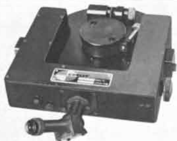
unisec positions precise guidance equipment in missiles prior to launching
