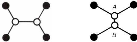
Two stable soap-film trees for four points on a rectangle. Only the left tree is minimal
